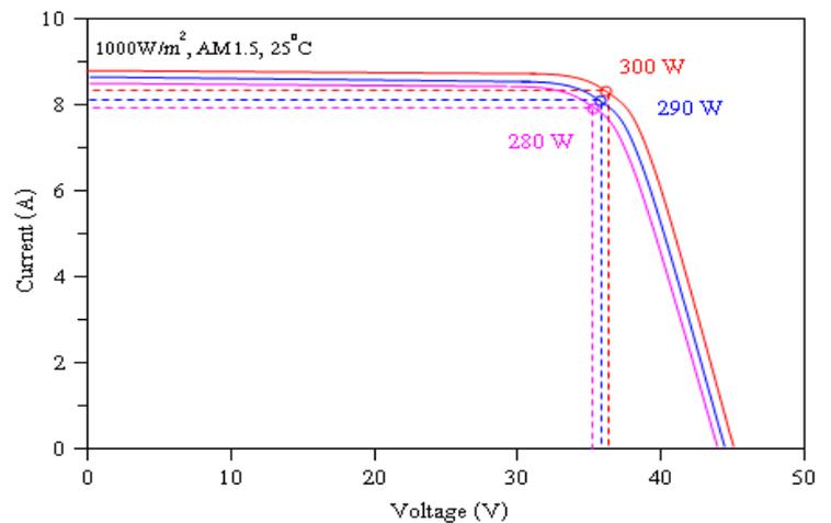
Electrical specification are based on measurements performed at standard test conditions (STC) of 1000 W/m<sup>2</sup> irradiance, air mass 1.5 and cell temperature of 25°C after long-term stabilization. Performance may vary up to 10% from rated power due to temperature operation, spectrum and related effects.
