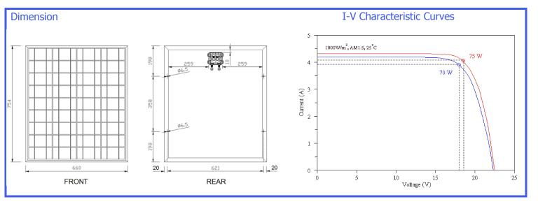
Electrical specification are based on measurements performed at standard test conditions (STC) of  $1000 \text{ W/m}^2$  irradiance, air mass 1.5 and cell temperature of 25°C after long-term stabilization. Performance may vary up to 10% from rated power due to temperature operation, spectrum and related effects.
