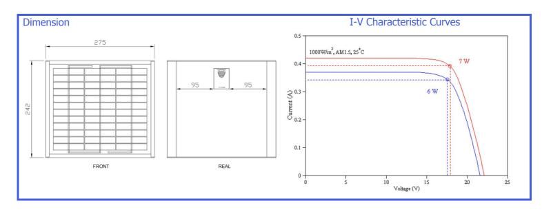
Electrical specification are based on measurements performed at standard test conditions (STC) of  $1000 \text{ W/m}^2$  irradiance, air mass 1.5 and cell temperature of  $25^{\circ}$ C after long-term stabilization. Performance may vary up to 10% from rated power due to temperature operation, spectrum and related effects.
